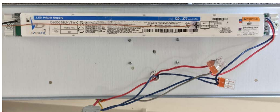
Figure 4. View of In-situ Point – Tc1 for LED driver of light source
